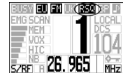
SQ knob is inactive. Remote SQ (=digital threshold) is active (Remote squelch RSQ)
