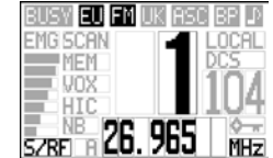
SQ knob is inactive. Remote SQ (=digital threshold) is active (Remote squelch RSQ)
